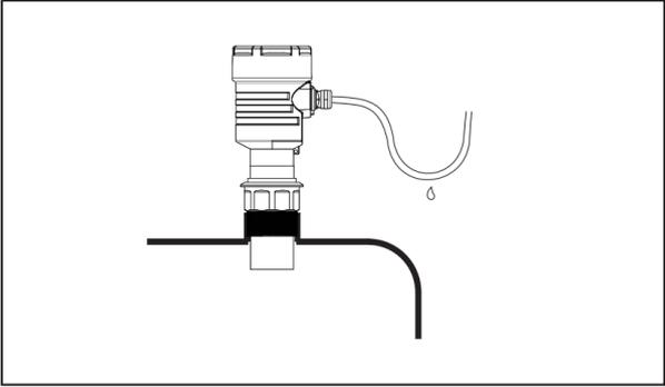
For sensors installed outdoors or in damp rooms and on cooling or heated tanks, the cable seal should be tightened to prevent moisture and the cable should be bent downward at the inlet. As shown below:
