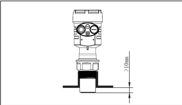
Length of container nozzle: Ensure that the probe extends out of the nozzle at least 10mm
