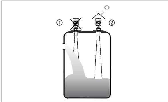
1 Not OK: Do not install the meter above the feed flow to ensure that you are measuring the surface of the medium and not the feed flow.
