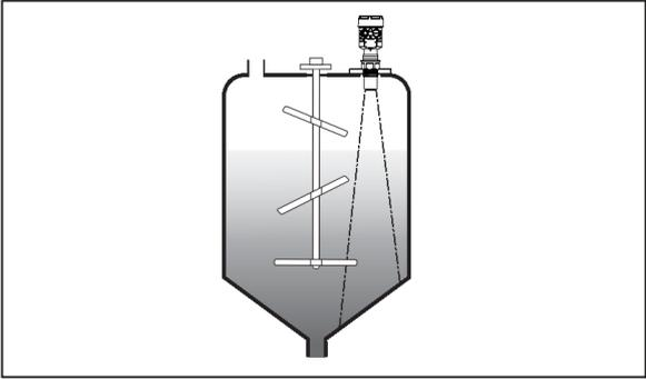
When there is stirring in the tank, the meter is installed as far away from the mixer as possible. After installation, "false echo learning" should be carried out in the stirred state to eliminate the false echo influence generated by the stirred blade. If foam or waves are generated due to stirring, wave guide tube installation should be used.
