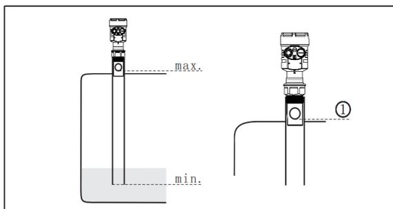
1 The diameter of the air hole (5~10) mm is installed using a guided wave tube (guided wave tube or bypass tube), which can avoid the influence of obstacles, foam and air eddy current in the container.
