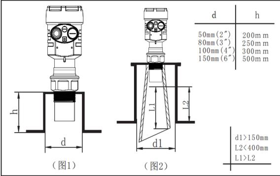
In the case of good reflection characteristics of the medium, when the diameter of the container nozzle is large, the nozzle length can be slightly longer than that of the transducer (figure 1).
