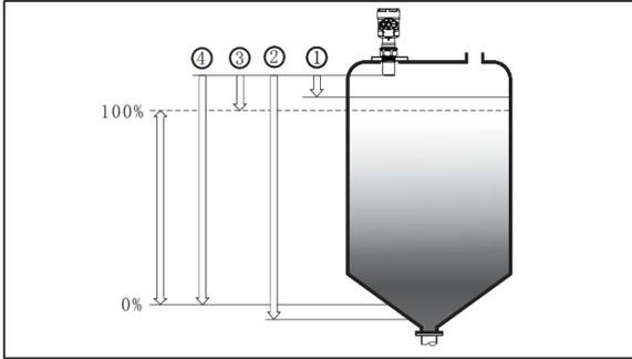
The datum for measurement is the lower edge of the probe.
