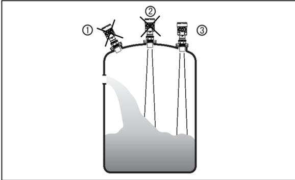
1 Not OK: The sensor should be perpendicular to the surface of the measured medium.
