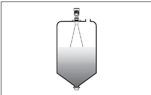
For conical containers with flat tops, the best place to install the meter is in the center of the top of the container, which ensures measurement to the bottom of the container.
