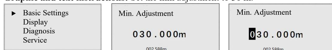
**Meaning of the parameter:** The min adjustment corresponds to the empty position, as shown in the following figure.
