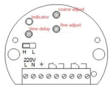
1. For an empty container, if the indicator is red light, rotate the fine adjust button counterclockwise till it turns into green, and then continue rotate for  $30^{\circ}$  counterclockwise, instrument will be ok to use then. If any problem during adjust, please contact with us.
